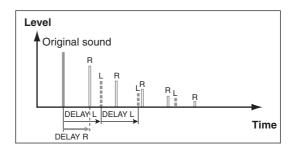
This effect adds two delayed sounds; one each for the L and R channels. You can control each delay independently. Each aspect of the sound is controlled by the following effect parameters.
