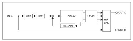
This effect adds delayed sounds to the Left, Center, and Right channels. Each delay can be controlled independently. Each aspect of the sound is controlled by the following effect parameters.
