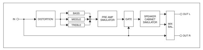
This effect simulates the characteristics of a guitar amp. Previously when recording an electric guitar in a studio, it was usual to play the guitar through an amp and then mic the amp in order to obtain the tonal character typical of the amp. This effect simulates the result without requiring you to use an amp.
